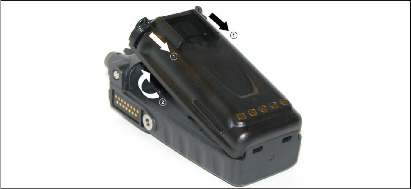
**Figure 4-1: Removing the Battery Pack**
