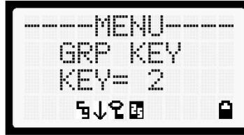
**Figure 8-5: Group/Channel Encryption Key Display**
